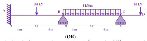
10. Analyze the Continuous beam as shown in figure using Stiffness method
