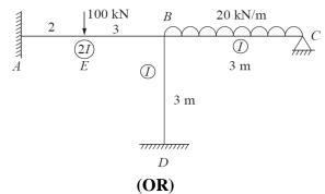
4. Find the support moments at A, B, C and D for the portal frame by using Moment **14M** Distribution Method shown in fig
