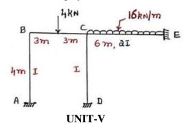
9. Determine the horizontal deflection of joint B as shown in fig below. Take 14M E=200 kN/mm<sup>2</sup>. Take A = 600 mm<sup>2</sup> for all the members. Using Castigliano's theorem.
