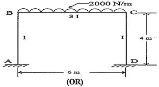
Analyse the portal frame given in figure by Moment distribution method.
